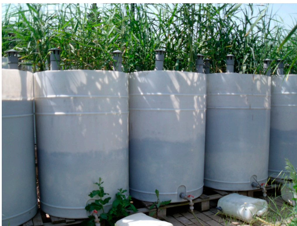
Figure 7. Picture of the pilot STRB in Xanthi (northern Greece) treating activated sludge with a high Cr content.
